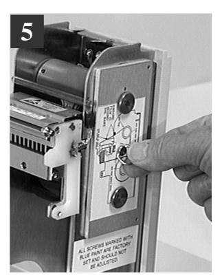
Turn the 'Dzus' Fastener 1/4 turn clockwise to lock in place. Lay the ring flat against the panel
